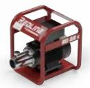
REDLINE RD22E Operating mass: 28 kg Battery type: Electrical single phase Manufacturer/Power: Branded / 2.2 kW @ 2800 rpm
