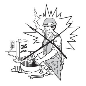
Never use petrol for cleaning purposes. Store inflammable or hazardous substances in well-sealed vessels when they are not in use. Wear appropriate face mask when using hazardous substances.
