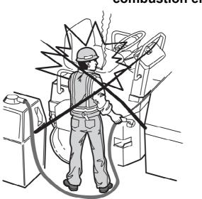
5. Refueling (machines with combustion engine)
